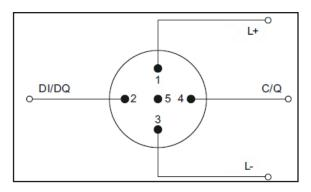
Figure 4: Pin assignment Port Class A
