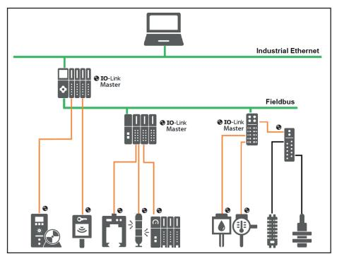
Figure 1: Example of system architecture with IO-Link
