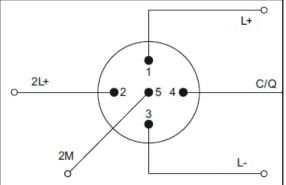
Figure 5: Pin assignment Port Class B
