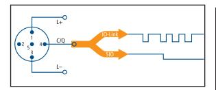
Figure 3: Pin assignment of IO-Link device
