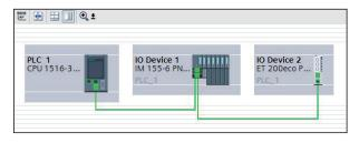
Figure 7: Configuration of a PROFINET network with lower-level IO-Link masters
