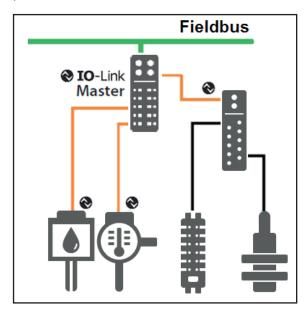
Figure 2: IO-Link point-to-point connection
