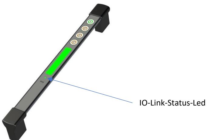
A status LED is clearly visible on the signaling device. This status LED shows the IO-LINK status in GREEN during normal operation. If device errors are detected with the integrated self-diagnosis, the IO-LINK status changes to RED.
