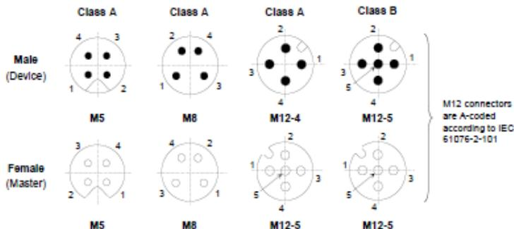
Port Class A (type A): With this type, the functions of pins 2 and 5 are not predefined. These functions are defined by the manufacturer. Pin 2 can be assigned an additional digital channel.
